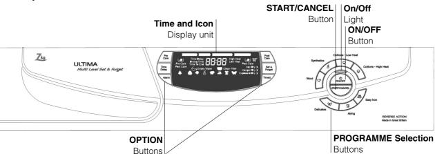
The **START/CANCEL** button starts a selected programme. When you press this button there will be one short beep and the progress icons will flash on/off to confirm the action. If you have not set a programme, the buzzer will beep four times. When a programme is running, holding this button in gives one long beep and cancels the programme and stops the dryer (see Start and Programmes).
